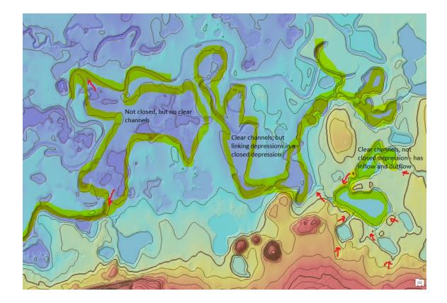
B. Delineating watersheds around the depressions can also help identify if there is connectivity out of the depression to a stream channel.
