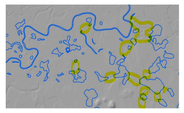
B. Geomorphic derivatives may be used to identify a channel. In this example, channels were found using geomorphic derivatives that do not enforce flow. BotHat channels, curvature and geomorphons were run on the unaltered surface. The pink (BotHat channels, Red (curvature) and green (geomorphon valleys and depressions) indicate more natural connections between features.
