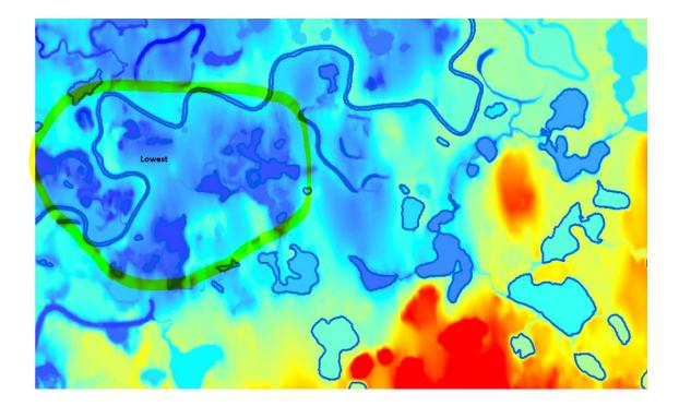
B. To understand general flow direction, a flow direction raster that is not hydro enforced (no fills) can be made. This will show the surface flow without forcing the flow to be connected throughout the watershed. Arrows show direction of flow based on elevation surface. Vectors of flow from multiple directions into depressions often indicate an isolated depression.
