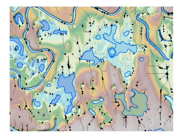
Consideration 4: Identify depressions nested inside of closed depressions. These do not need to be connected even if there are clearly identifiable channels between the inner depressions:
