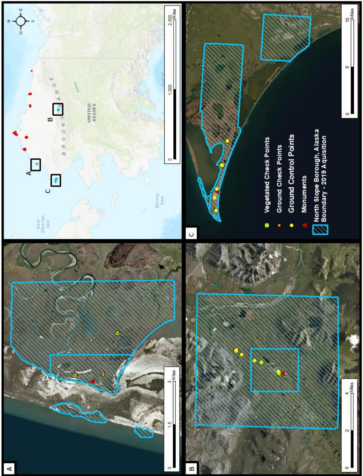
Figure 3b: Ground survey location map – 2019 Acquisition
