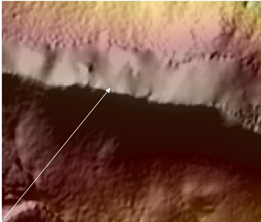
Figure 4 - Tiles N5145E17945P and N5145E17930P from cell 416. Loss of surface definition is generally present in areas of steep terrain where interpolation methods were used to fill void areas.
