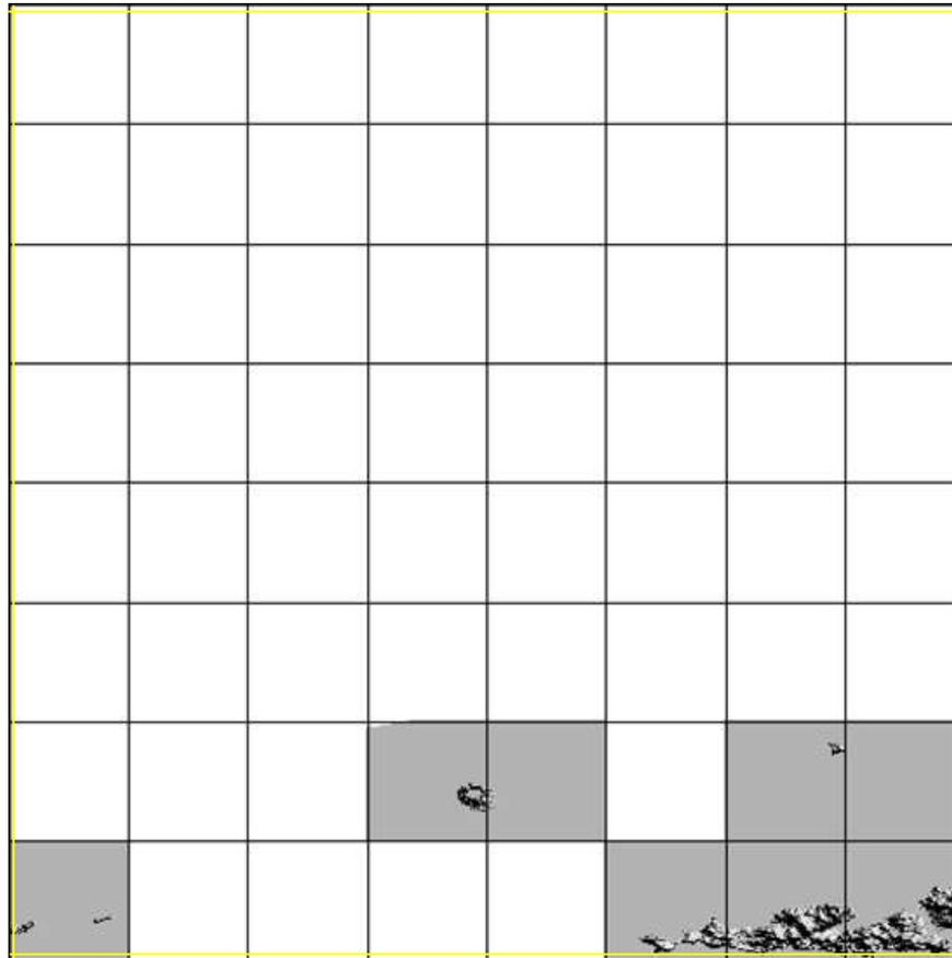
Tile edges were checked visually for matching elevation values and seam lines in the DTM and DSM
