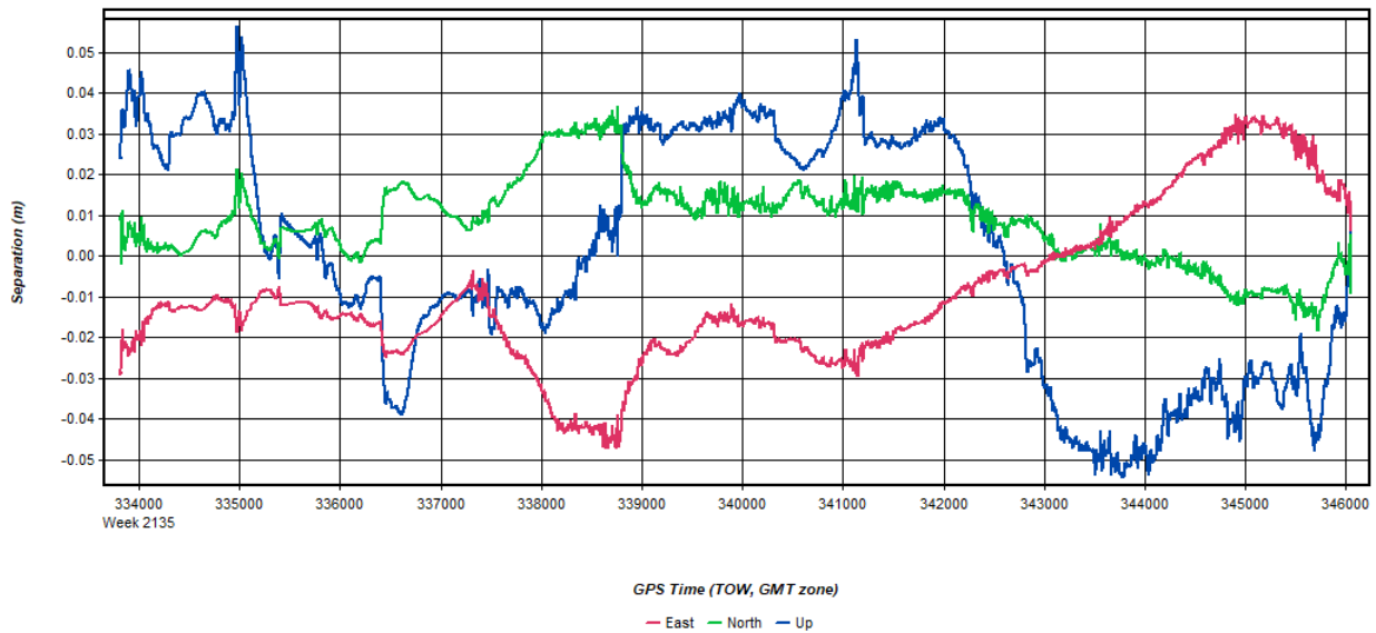
Figure 2: 20201209203945_2 [Smoothed TC Combined] - Forward/Reverse or Combined Separation Plot
