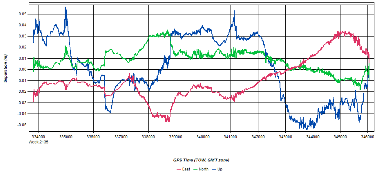
Figure 4: 20201209203945_2 [Smoothed TC Combined] - Forward/Reverse Separation Plot (Fixed)
