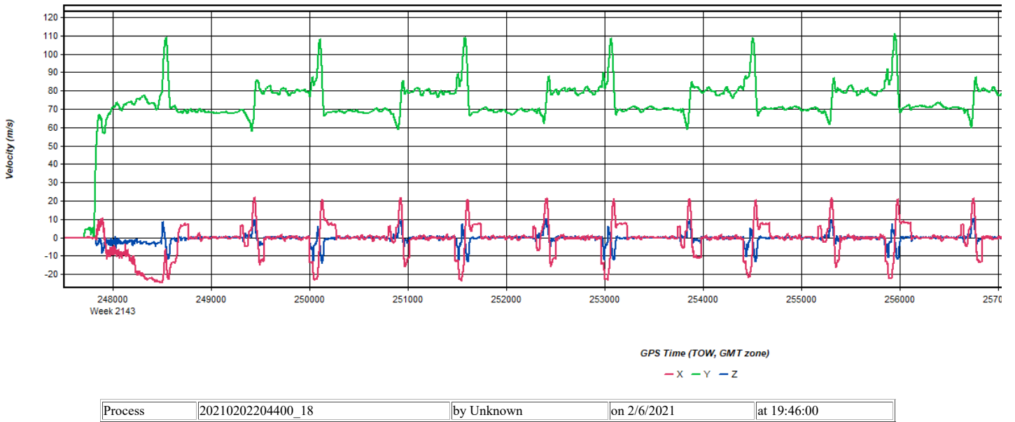
Figure 14: 20210202204400_18 [Smoothed TC Combined] - Body Frame Velocity Plot
