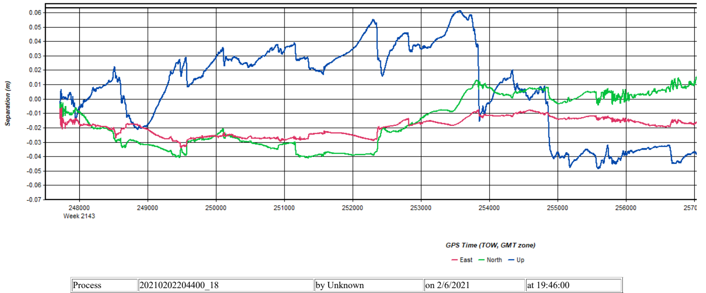
Figure 4: 20210202204400_18 [Smoothed TC Combined] - Forward/Reverse Separation Plot (Fixed)
