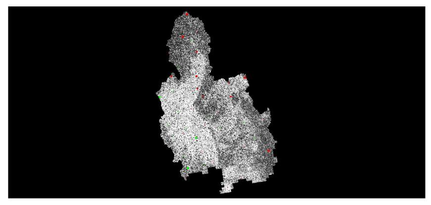
Green represents where the lidar surface is above the check point (positive elevation error).
