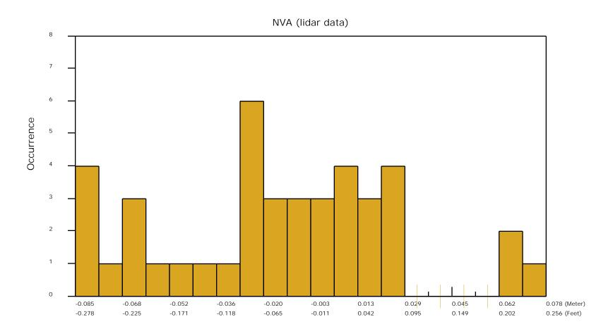
The purpose of this section is to show a frequency distribution chart of the vegetated vertical accuracy (VVA) of the lidar point cloud data measured against surveyed ground check points.
