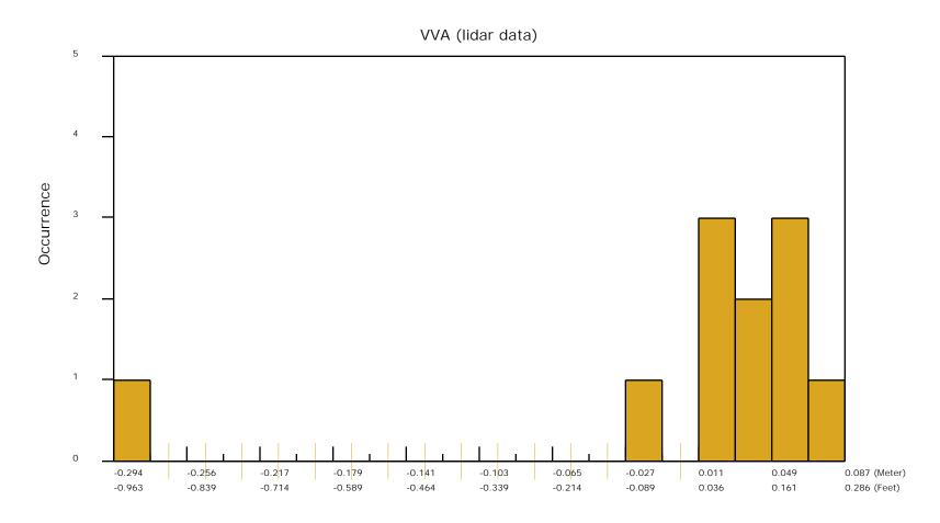
The purpose of this section is to show a frequency distribution chart of the non-vegetated vertical accuracy (NVA) of the DEM data measured against surveyed ground check points.
