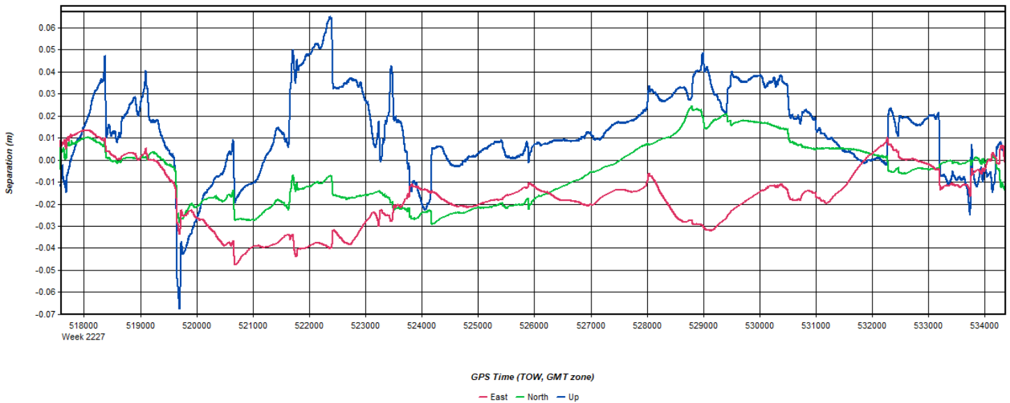
Figure 2: 20220916234534_4 [Smoothed TC Combined] - Forward/Reverse or Combined Separation Plot
