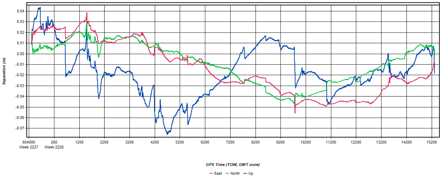
Figure 2: 20220917234411_6 [Smoothed TC Combined] - Forward/Reverse or Combined Separation Plot
