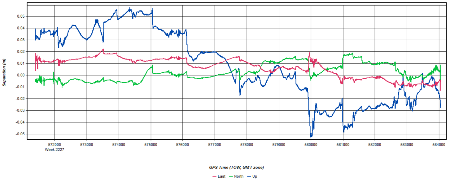
Figure 2: 20220917143805_5 [Smoothed TC Combined] - Forward/Reverse or Combined Separation Plot
