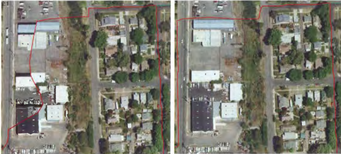
Seamlines before (left) and after (right) correction of seamline cutting through building.
