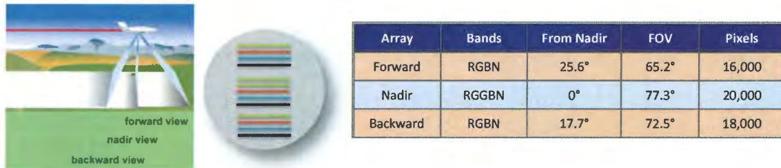
ADS100 imaging operations (Courtesy Leica Geosystems).
