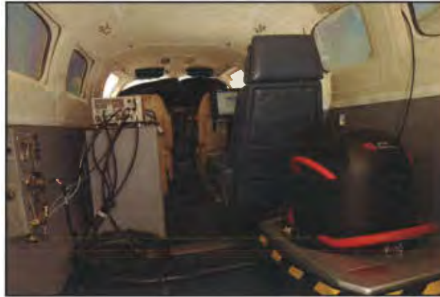
ADS100 Installation in a Surdex Cessna 441 (Conquest) Aircraft.
