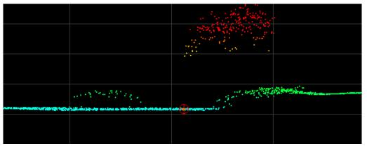
Figure 8 – Non-vegetated checkpoint NVA-69 shown as the large red marker is located underneath a tree. This point was removed from raw swath vertical accuracy testing because above ground features including trees have not been separated from the ground classification yet.
