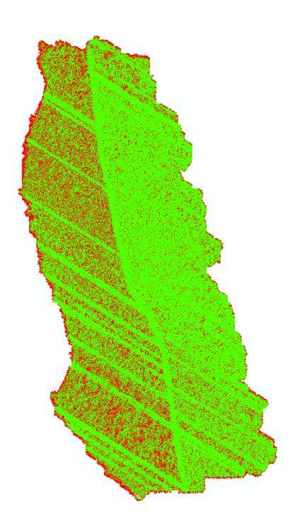
Figure 17– 1-square meter density grid. There are some 1-meter cells that do not contain 8 points per square meter (red areas) due to the irregular spacing of lidar point cloud data. Most 1-square meter cells contain at least 8 points per square meter (green areas) showing there are no systematic density issues. When density is viewed/analyzed by representative 1-square kilometer areas density passes with no issues.
