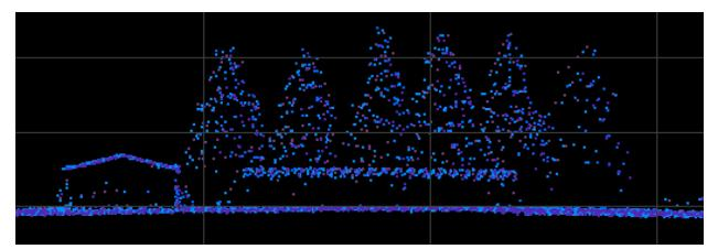
Figure 16– Horizontal Alignment. Two separate flight lines differentiated by color (Teal/Purple) are shown in this profile. There is no visible offset between these two flight lines. No horizontal alignment issues were identified.
