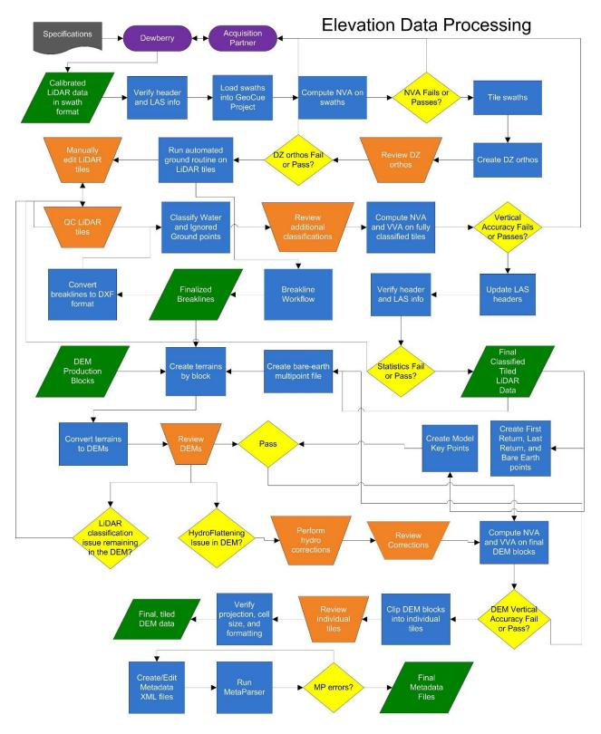
Figure 29-DEM Production Workflow
