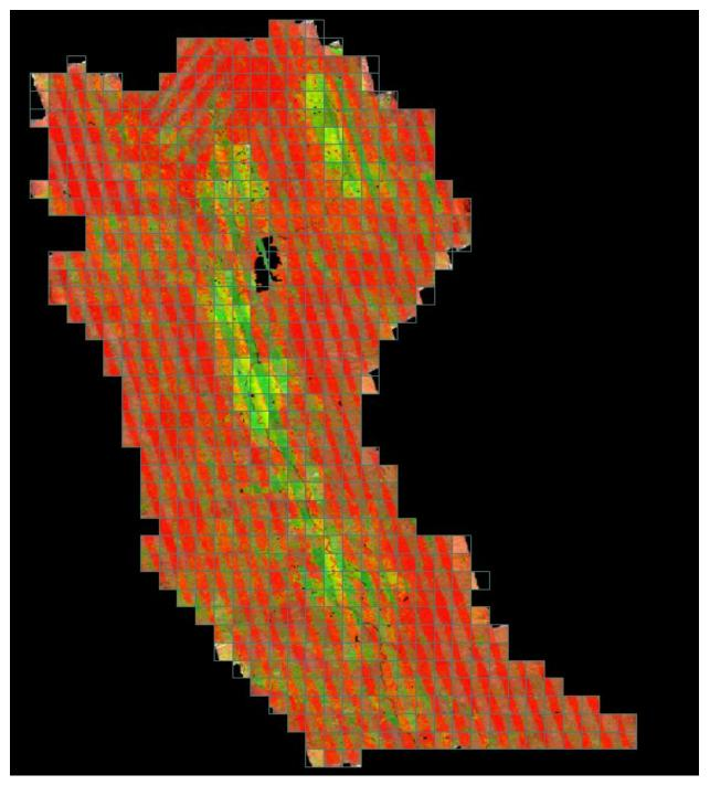
Figure 12-- Single return DZ Orthos for the Russian Mendocino AOI. Heavy vegetation obscured much of this AOI so additional verifications were performed. Open, flat areas are shown in green as they meet specifications. Inter-swath relative accuracy passes specifications.
