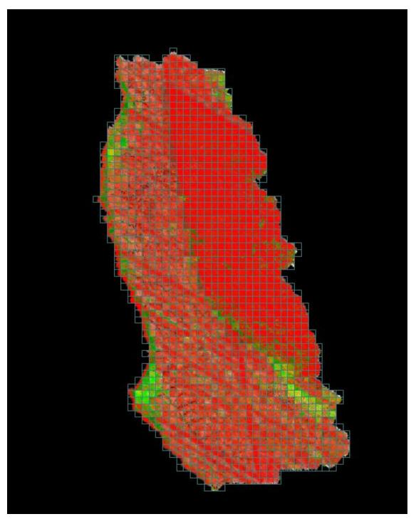
Figure 9-Single return DZ Orthos for the Mendocino QL1 AOI. Heavy vegetation obscured much of this AOI so additional verifications were performed. Open, flat areas are shown in green as they meet specifications. Inter-swath relative accuracy passes specifications.
