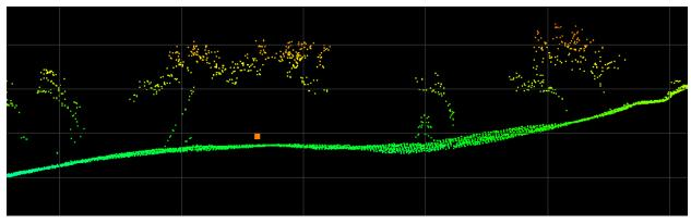
Figure 24 – VVA-35 shown as the orange square in the profile is located 6+ feet above the actual ground surface. This checkpoint was removed from all vertical accuracy calculations due to incorrect survey.
