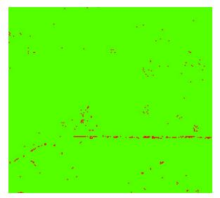
Figure 19– Spatial Distribution. All cells (2\*NPS cellsize) containing at least one lidar point are colored green. Cells that do not contain a lidar point including water bodies which are acceptable NoData area are colored red. Without removing acceptable NoData areas due to water 98% of cells contain at least one lidar point.
