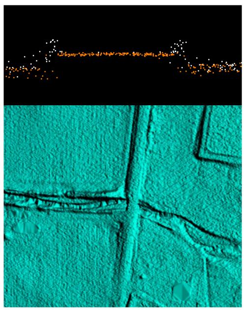
Figure 22– Tile number 10SDJ854280. Profile with points colored by class (class 1=white class 2=orange) is shown in the top view and the DEM is shown in the bottom view. This culvert remains in the bare earth surface. Bridges have been removed from the bare earth surface and classified to class 17
