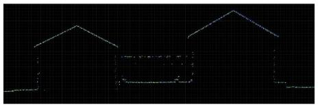
Figure 7 – Profile views showing correct roll and pitch adjustments.
