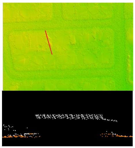
Figure 20 – Tile number 10SDJ823325. Profile with points colored by class (class 1=white class 2=orange) is shown in the bottom view and a TIN of the surface is shown in the top view. The cross section identifies a low porch. A limited number of these small features are still classified as ground but do not impact the usability of the dataset.
