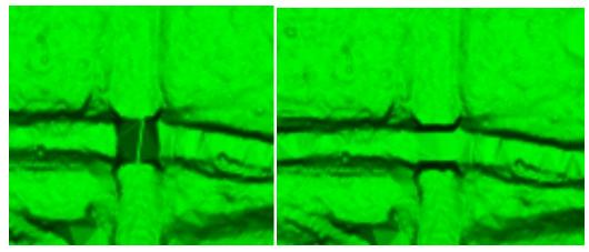
Figure 32- DEM on the left shows a bridge saddle artifact while the DEM on the right shows the same location after Bridge saddle breaklines have been enforced.
