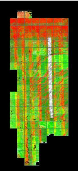
Figure 13-- Single return DZ Orthos for the Cow Creek AOI. Inter-swath relative accuracy passes specifications.
