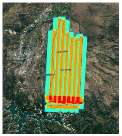
Figure 6 - Lidar swath output showing complete coverage for Cow Creek
