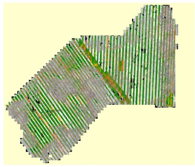
Figure 10- Single return DZ Orthos for the Upper Pit AOI. Inter-swath relative accuracy passes specifications.
