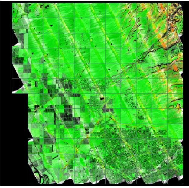
Figure 11- Single return DZ Orthos for the Keefer Slough AOI. Inter-swath relative accuracy passes specifications.
