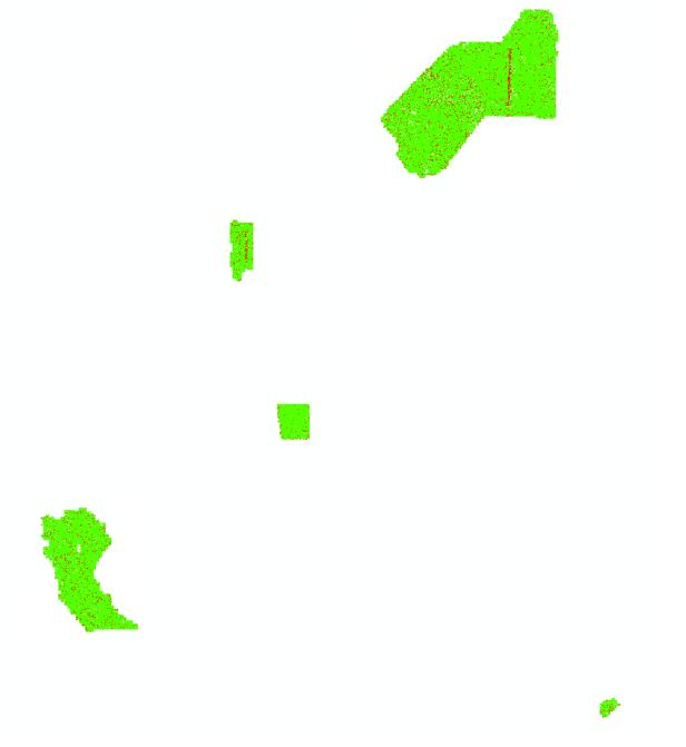
Figure 18– 1-square meter density grid. There are some 1-meter cells that do not contain 2 points per square meter (red areas) due to the irregular spacing of lidar point cloud data. Most 1-square meter cells contain at least 2 points per square meter (green areas) showing there are no systematic density issues. When density is viewed/analyzed by representative 1-square kilometer areas density passes with no issues.
