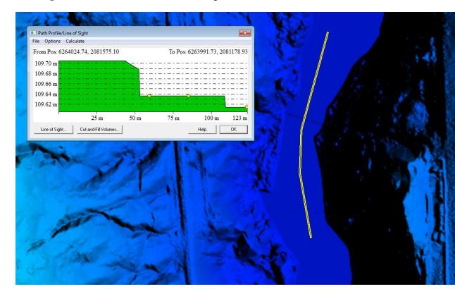
Figure 23 – Tile number 10SDJ948022. Elevation change has been stair stepped. The steps are flat from bank to bank and flow consistently downhill.
