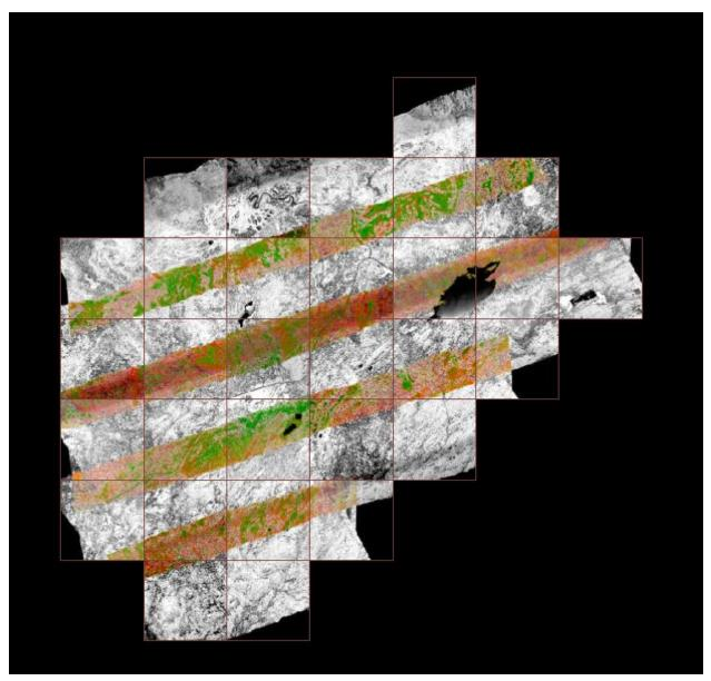
Figure 14-- Single return DZ Orthos for the Alpine AOI. Inter-swath relative accuracy passes specifications.
