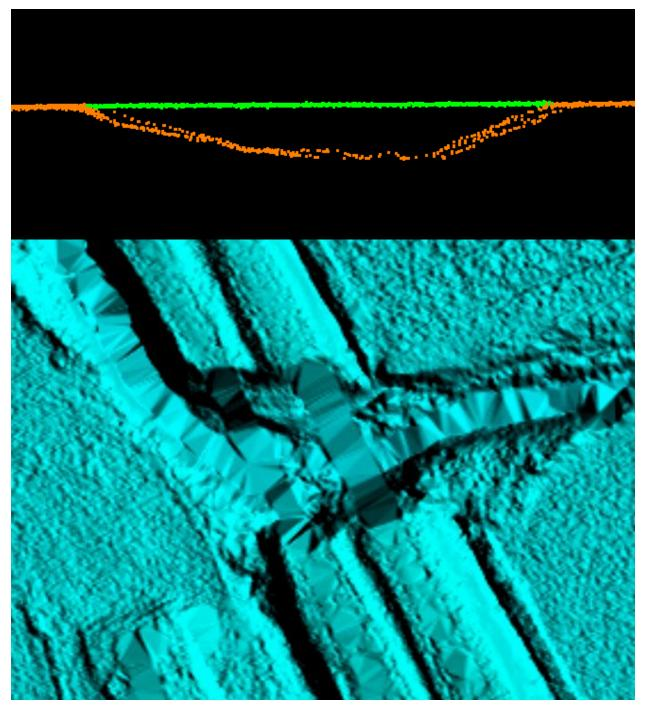
Figure 21 – Tile number 10SDJ823264. The DEM in the bottom view shows an area where a bridge has been removed from ground. The surface model must make a continuous model and in order to do so points are connected through interpolation. This results in less detail where the surface must be interpolated. The profile in the top view shows the lidar points of this particular feature colored by class. All bridge points have been removed from ground (orange) and are bridge deck (green).
