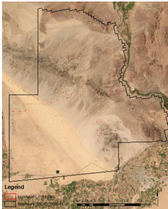
Figure 8. Intraswath polygons used to test intraswath vertical accuracy
