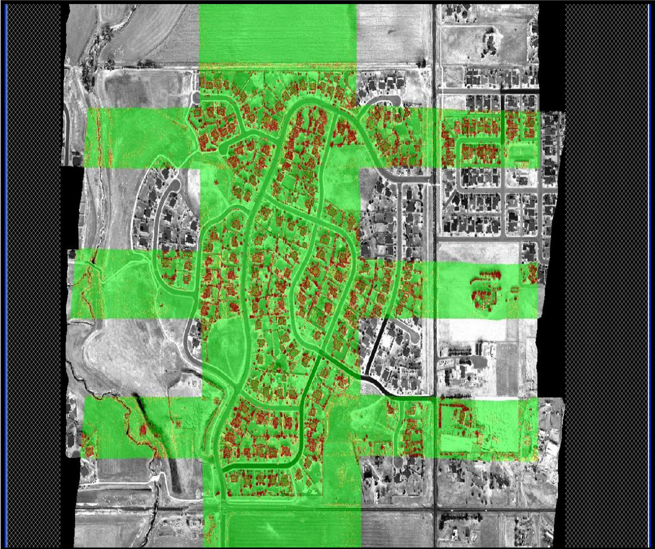
MARS® tests for internal relative vertical accuracy using inbound and outbound scan values. Again, Green is showing inbound and outbound scan data fitting to 3 centimeters.
