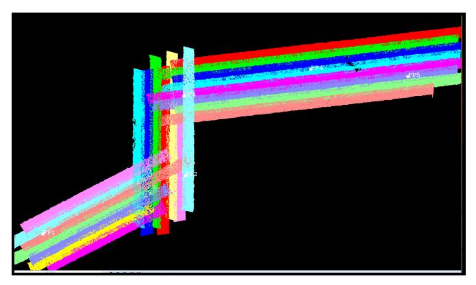
The next step is to match the ground control elevations to the lidar data set. A control report is run and the data set is shifted slightly to zero out the average elevation error and points checked for quality.
