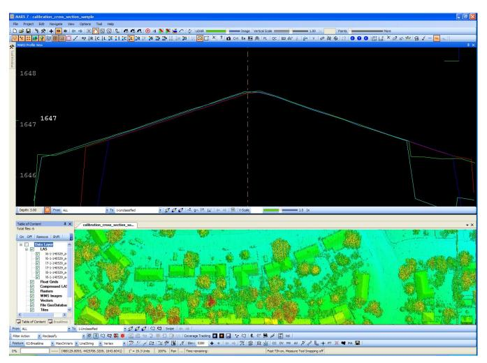
Roll and scale are checked on roof planes perpendicular to the flight direction.
