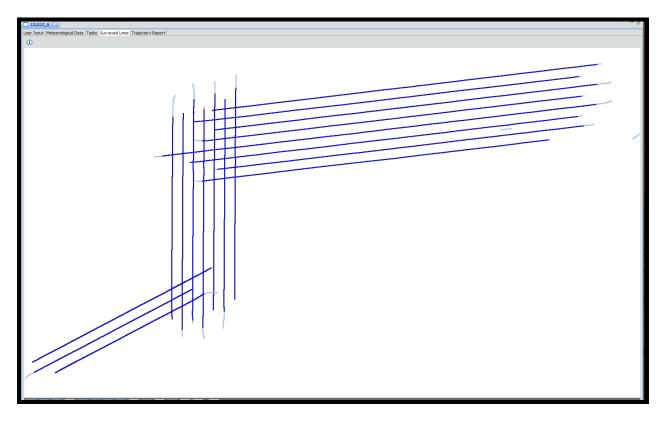
As in self-calibration the LMS production program analyses ground, roof planes and rooflines. One cross flight is locked in elevation and all other lines are adjusted to it. Unlike the calibration site the distribution of roof planes is usually much less dense. Here matched ground tie planes are blue.
