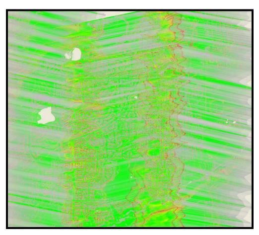
Plot of height differenced between flight lines. (Green=less than 5cm).
