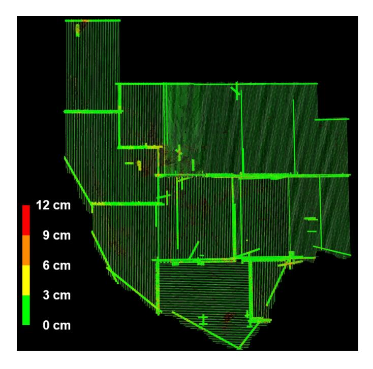
After boresighting is complete a detailed statistical report is generated to check relative and absolute accuracies before filtering of lidar begins. The calibration process yields excellent absolute accuracies, as can be seen for this example project.
