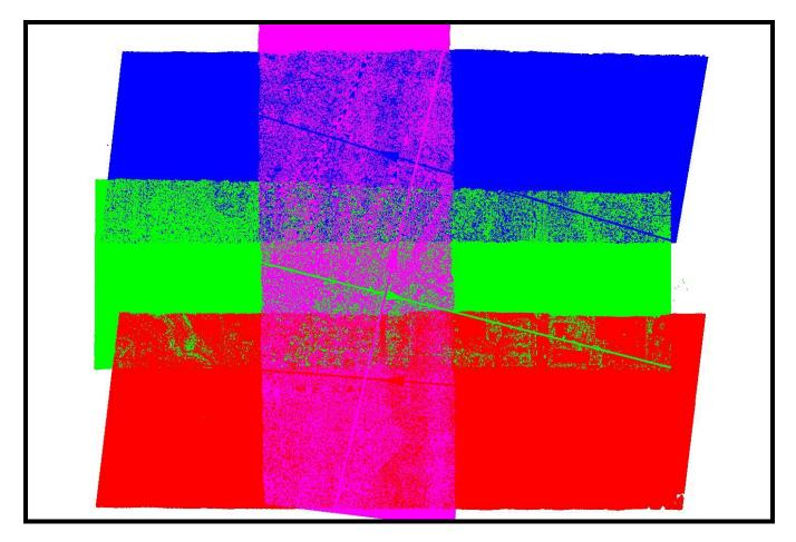
The Boresighting module frees scan angle scale, scan angle lag, XYZ boresight corrections and elevation position corrections while locking scan angle offset and XY position corrections.
