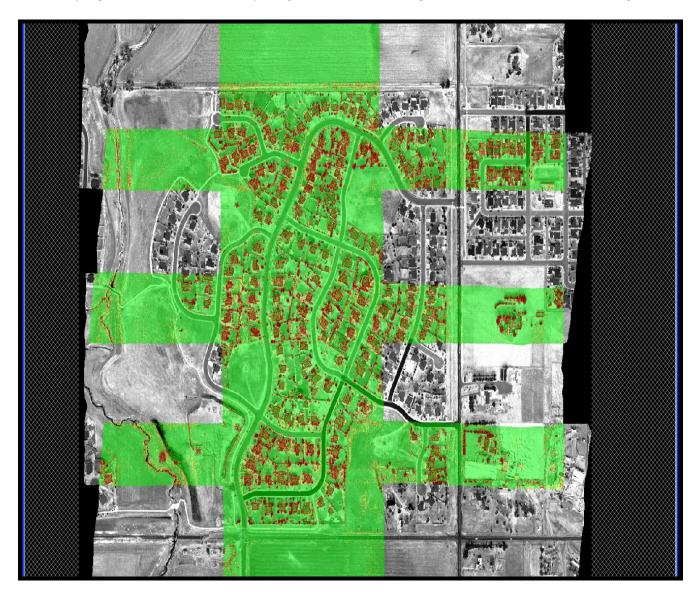
A Flight Line Separation Raster image is generated in Merrick Advanced Remote Sensing Software (MARS®), in this example ground returns from multiple flight lines that are fitting within 3 centimeters are colored green.
