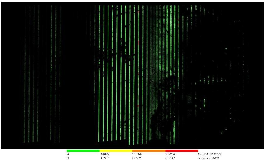
A maximum vertical separation cutoff has been applied to this graphic for the purpose of masking out disruptive features that do not show calibration issues between flight lines (e.g., trees, moving cars, etc.).
