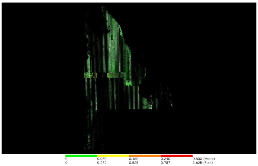
A maximum vertical separation cutoff has been applied to this graphic for the purpose of masking out disruptive features that do not show calibration issues between flight lines (e.g., trees, moving cars, etc.).
