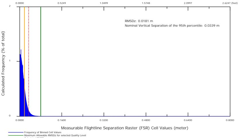
Frequency Distribution Chart of Measurable Flightline Separation Raster (FSR) Cell Values
