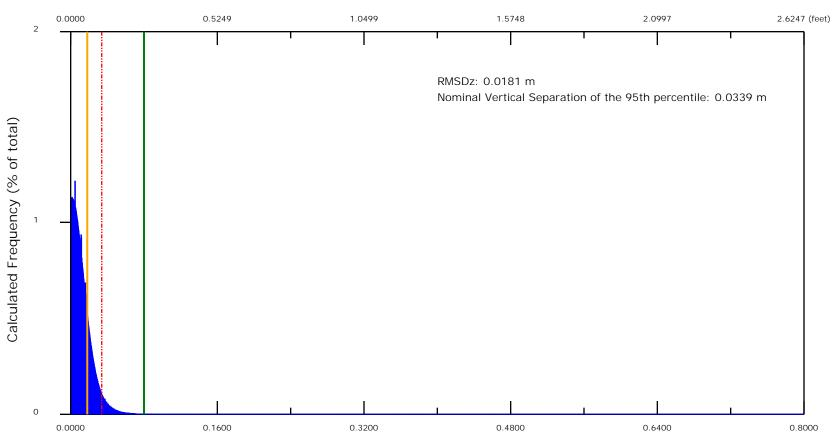
Measurable Flightline Separation Raster (FSR) Cell Values (meter)
