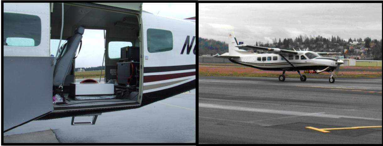
*The Cessna Caravan is a stable platform, ideal for flying slow and low for high density projects. A Leica ALS50ii sensor head installed in the Caravan is shown on the left.*
