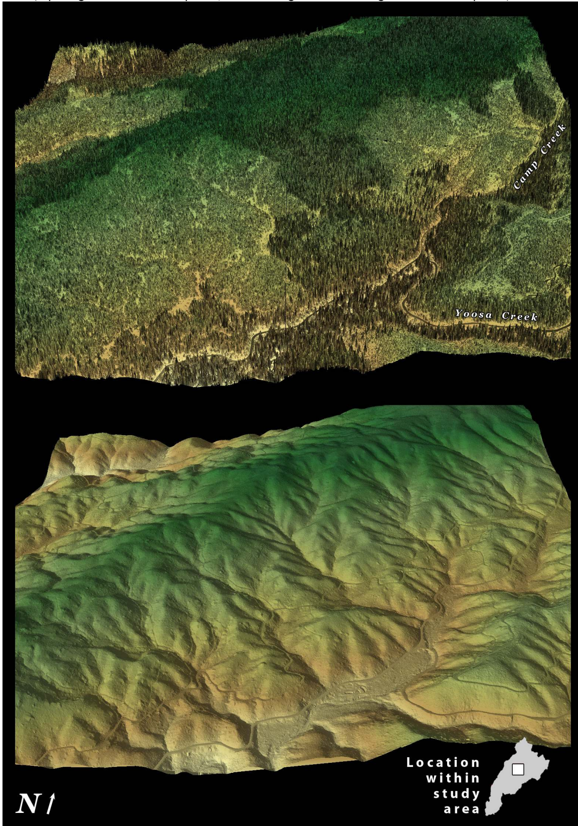
Figure 13. 3-d oblique view of LiDAR-derived surfaces in bins 29-30 and 39-40 of the Lolo Creek Study Area (top image derived from all points, bottom image derived from ground-classified points).
