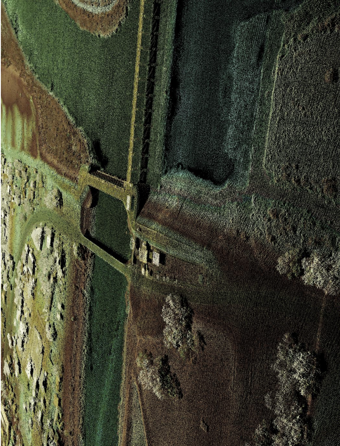
Figure 19: Image shows the Morelos Dam, looking north-northeast. The image was created from the bare earth model colored by elevation, and is overlain with the above-ground LIDAR point cloud.
