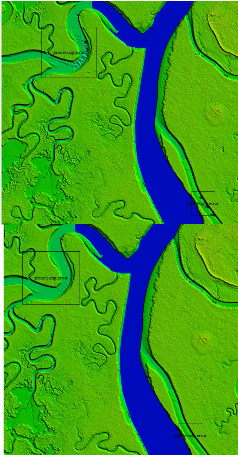
Figure 9- DEM_S23_3854_20. The above image is an overview of the DEM where USGS made two processing error calls. The below image is an overview of the reprocessed DEM with the processing error removed.
