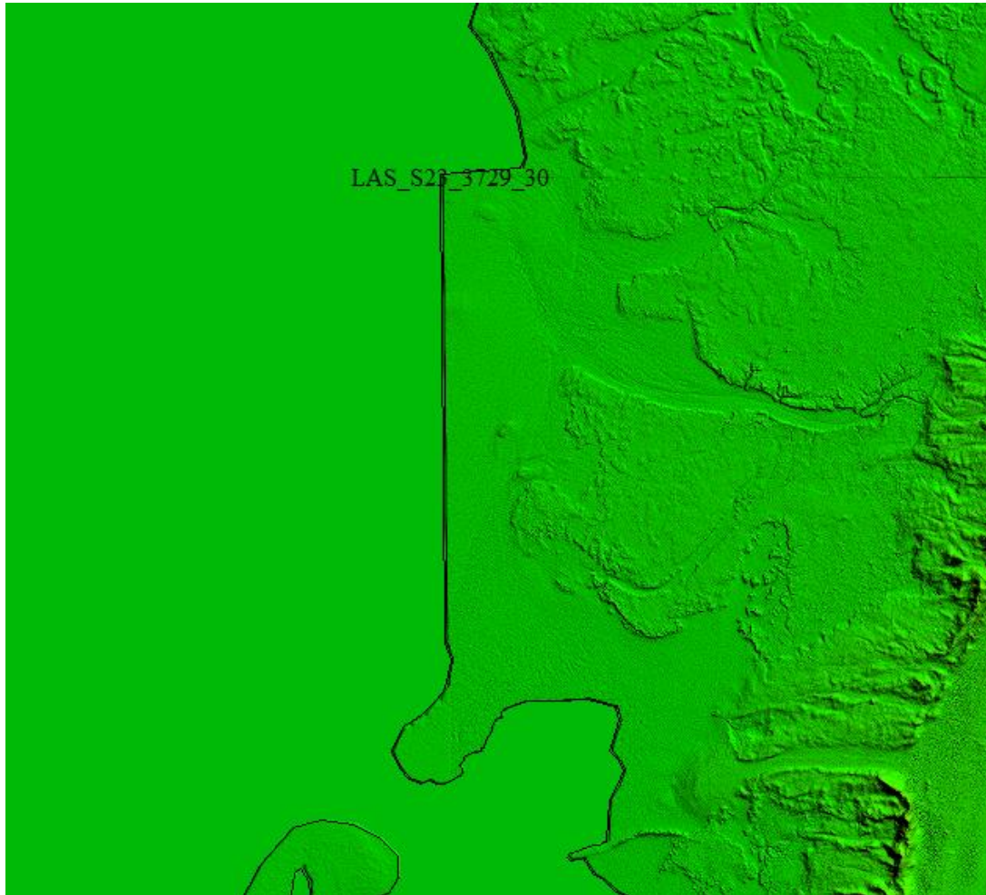
Figure 18- Tile DEM_S23_3729_30 shows a temporal difference where the Eastern Shore LEG data meets the Sandy data. The straight vertical line between the hydro flattened area and the terrestrial area is the dividing line between the Sandy topobathy data and the data collected by LEG. This area was submerged in the area collected by LEG and was not submerged in the Sandy data.
