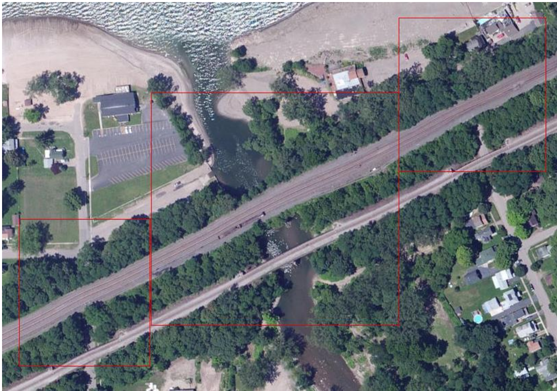
Figure 4 - Tile 17TPH565180. Bing Imagery shows that there are cinders/ ground between the railroad tracks and along the sides of the track. These three features are culverts and remain modeled in the ground surface.
