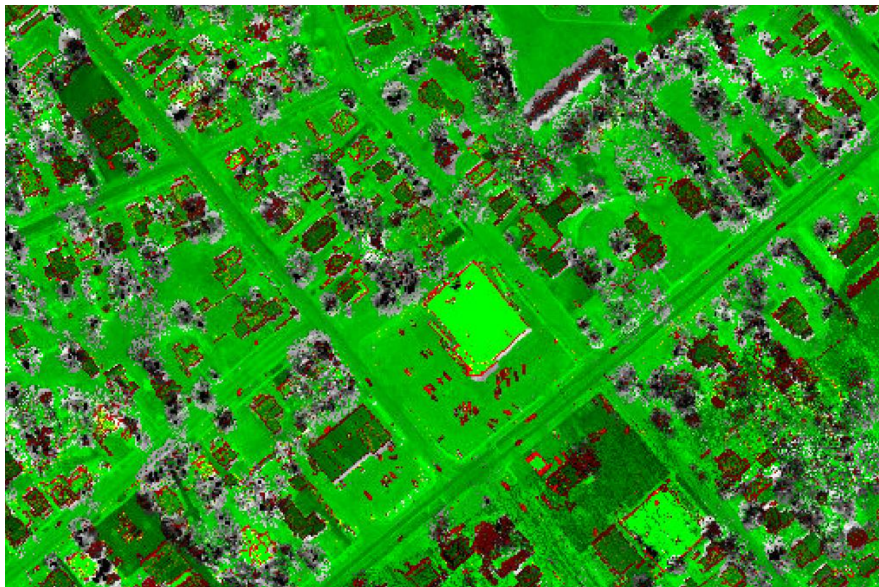
Figure 6 - DZ orthos created from the full point cloud. Some red pixels are visible along embankments, sloped terrain, building edges, and in vegetated land cover, as expected. Open, flat areas are green indicating the calibration and relative accuracy of the data is acceptable.
