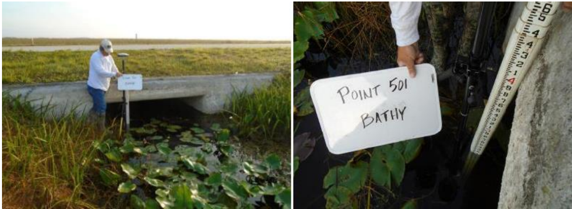
Figure 25 – Survey photos of bathy checkpoint 501 shown above. Bathymetric checkpoints 500 through 516 were removed from accuracy testing because they were determined to not be survey grade.
