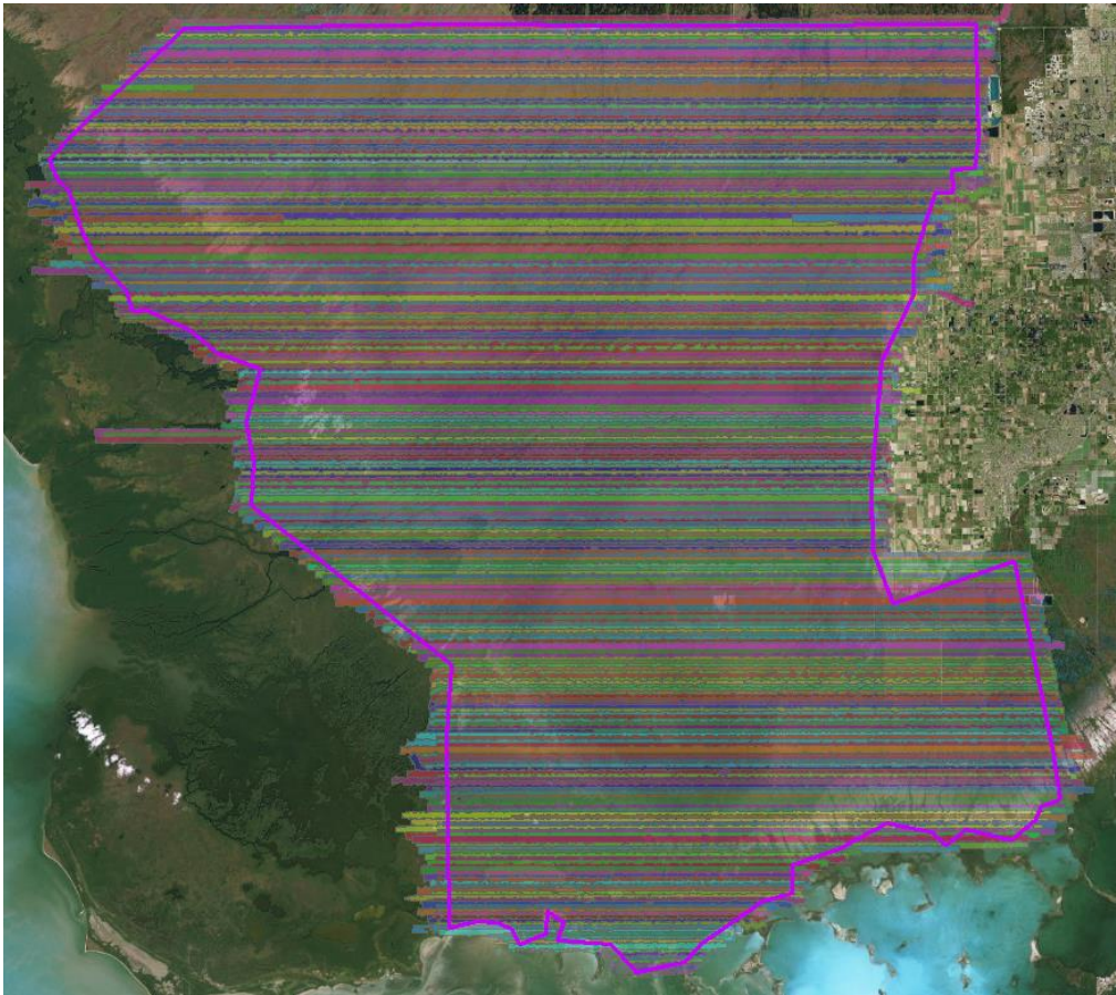
Figure 3 – Lidar swath output showing complete coverage.
