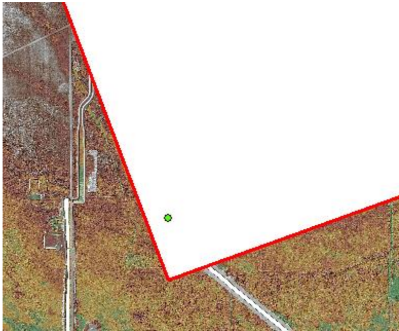
Figure 24 – Checkpoint NVA-413 (green) was removed from accuracy testing because it was located outside of the project boundary (red).
