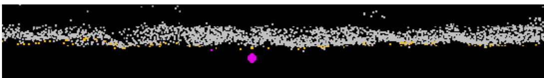
Figure 29 – VVA Point 239. The top two images show the dense vegetation at the survey tripod location. The lidar profile (bottom image) shows the lidar could not penetrate through the dense vegetation to the location of point 239 (pink).
