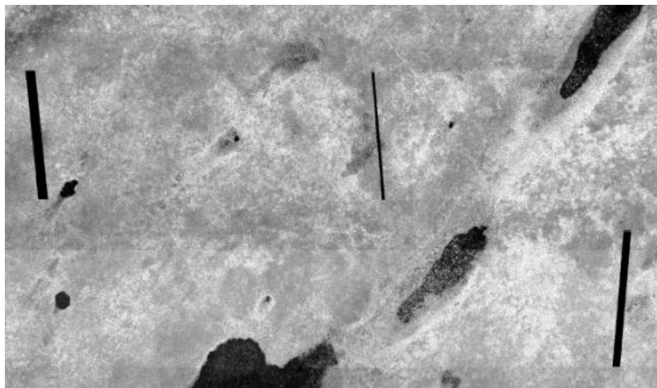
Figure 23 – The intensity imagery of the NIR sensor data contain small black strips in several localized areas. These strips are where drop-outs occurred during collection of the NIR data. This does not impact the coverage of the lidar and is only visible in the intensity imagery of the NIR sensor data. The Green sensor lidar data was combined with the NIR sensor lidar data to create complete coverage of the lidar point cloud. The combined data has been verified to meet project specifications. There are no detrimental effects to the DEM or any derivative products aside from the artifacts in the NIR intensity imagery.
