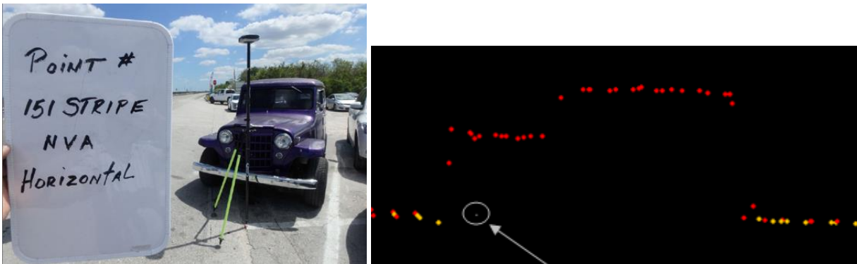
Figure 6 – Survey photo of NVA checkpoint 151 (left image) and profile view of the lidar with point location (right image). Checkpoint 151 is located underneath a parked vehicle. This point was removed from raw swath vertical accuracy testing because above ground features, including vehicles, have not been separated from the ground classification yet.
