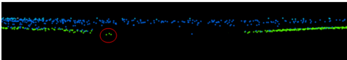
Figure 16 - Bathy Bottom points (green) are shown with water column (dark blue) and water surface points (light blue) in this profile. The four water column points circled in red would cause inconsistent and upward changes in the topobathy model if these points were classified to bathy bottom. These points should remain classified as water column.
