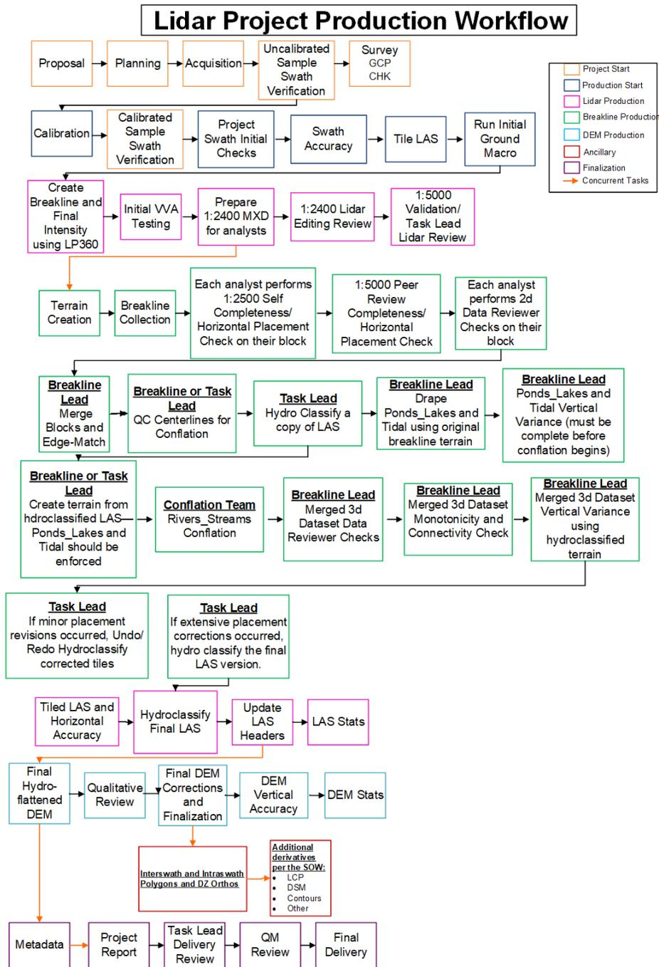
Figure 2 - Dewberry's lidar production workflow diagram.
