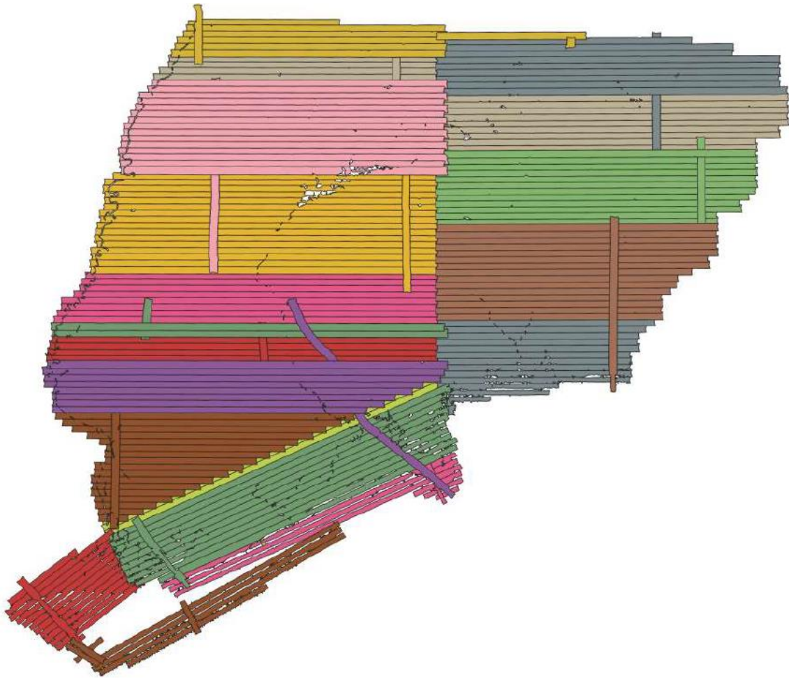
Figure 8 - Lidar swath output showing complete coverage.
