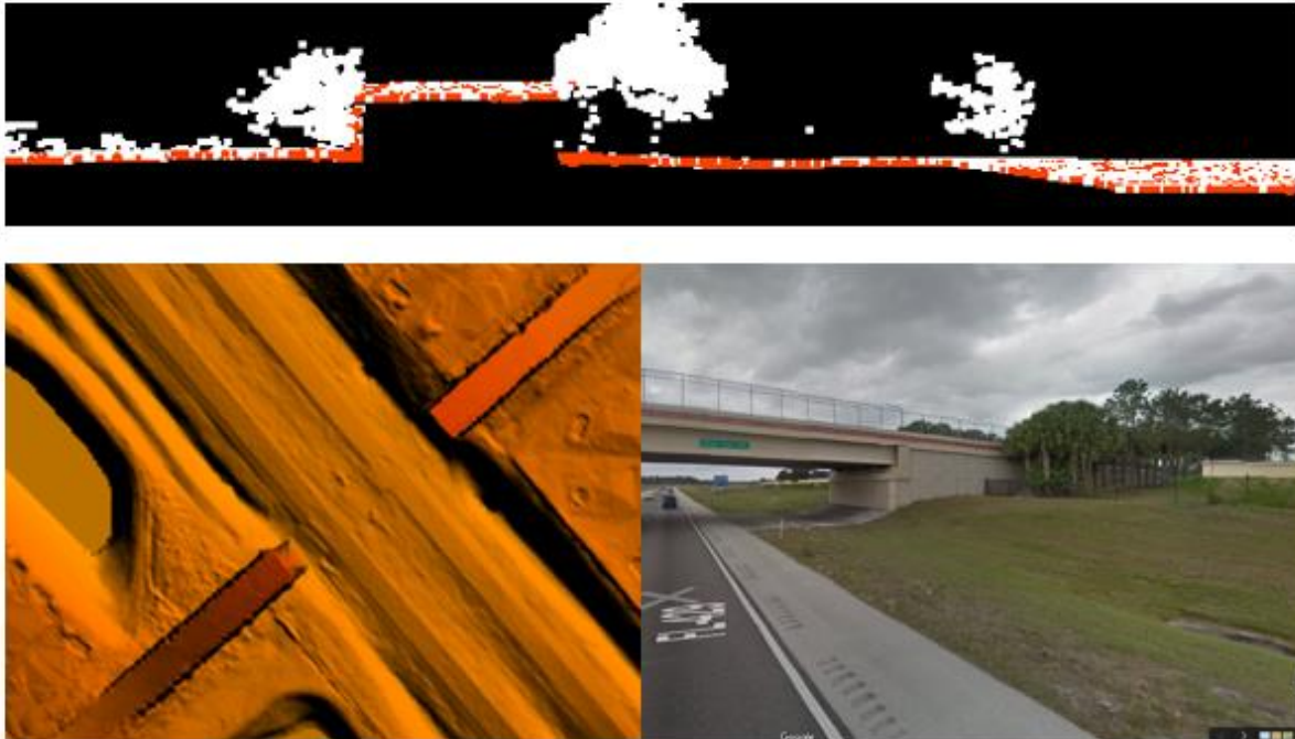
Figure 15– Tile LID2015_063158_E_B. Profile with points colored by class (class 1=white, class 2=orange) is shown in the top view, the DEM is shown in the middle and a google maps screenshot on the bottom. This area shows built up ground that resembles a bridge in the surface model. Only the actual bridge decks have been removed from the bare earth surface and classified to class 17.
