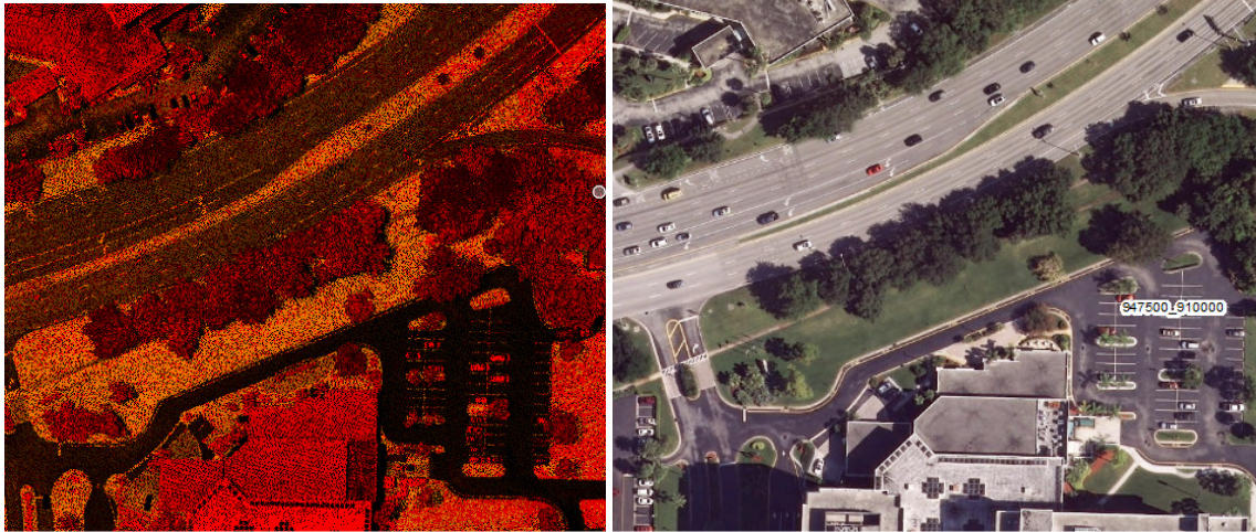
Figure 21 - Tile number 947500_910000. Full lidar point cloud (red=unclassified, orange=ground) is shown in the left image and orthoimagery of the same location is shown in the right image. This road and the parking lot are an area of low NIR reflectivity because the composition of the road materials result in the absorption of the NIR laser, reducing the number of lidar returns defining the road and the parking lot. Areas of low NIR reflectivity exist within this dataset.
