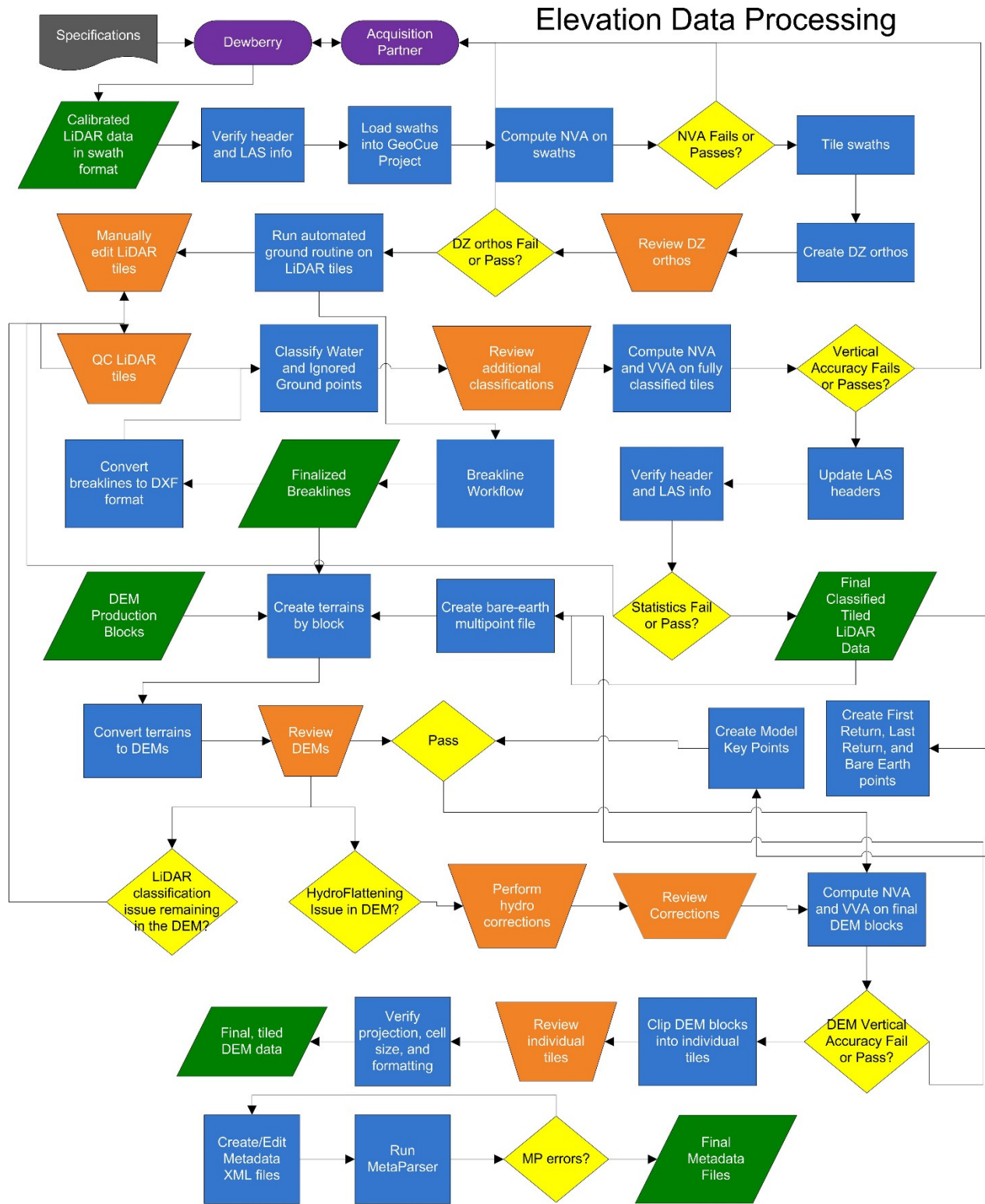
Figure 25 - DEM Production Workflow
