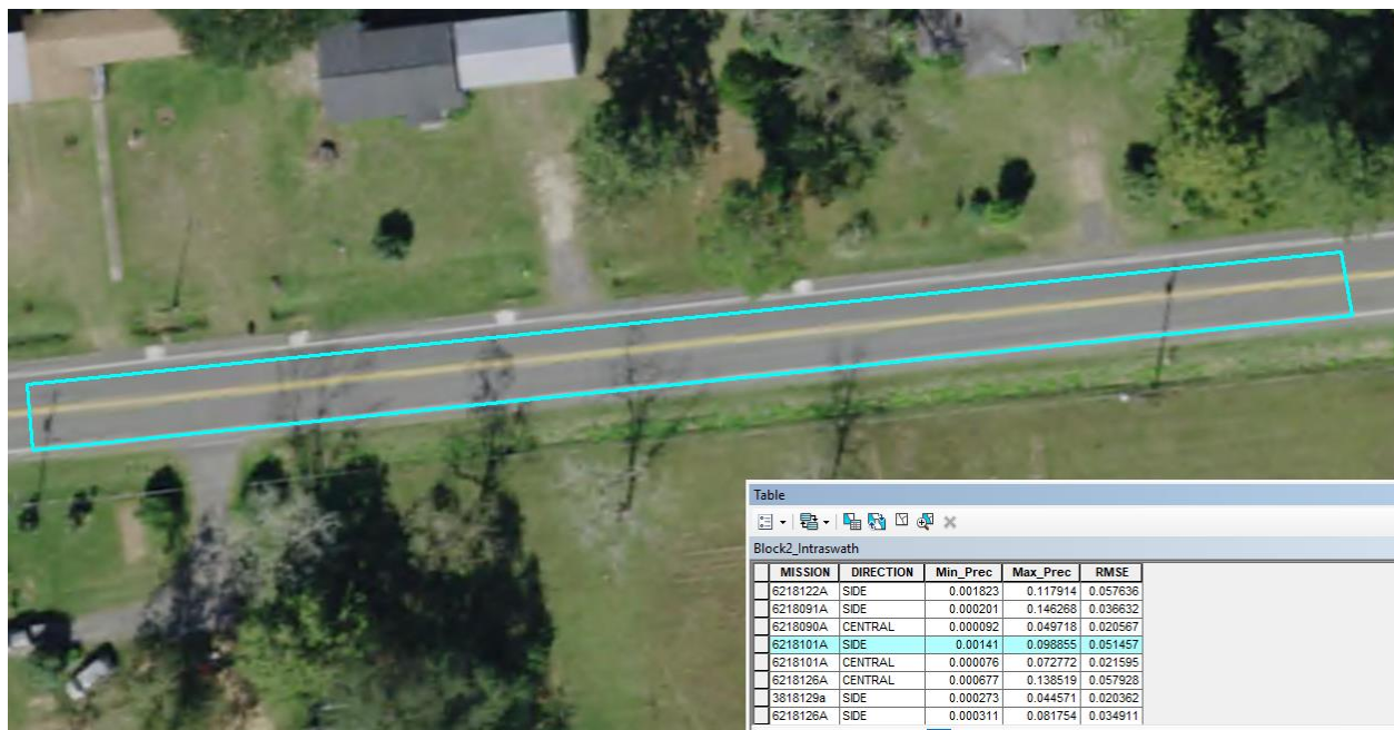
Figure 13—Example test polygon for intraswath testing, and its results.
