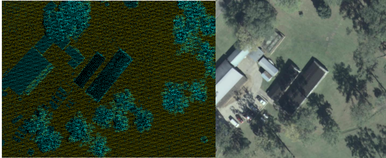
Figure 30-Tile number e1090n0081. Full lidar point cloud (cyan=unclassified, yellow=ground) is shown in the left image and orthoimagery of the same location is shown in the right image. The roof on the two buildings are areas of low NIR reflectivity because the composition of the roof materials result in the absorption of the NIR laser, reducing the number of lidar returns defining the roofs. Areas of low NIR reflectivity exist within this dataset.
