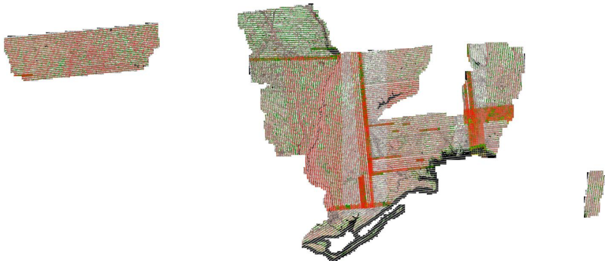
Figure 9– Single return DZ Orthos for the FL Panhandle LiDAR project. Inter-swath relative accuracy passes specifications.
