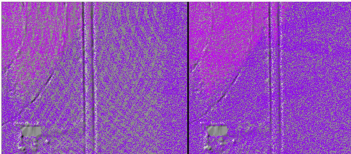
Figure 12 – The left image shows ground classified without synthetic points. The right image shows ground classified with synthetic points. Both images are overlaid on a hillshade of the example area.
