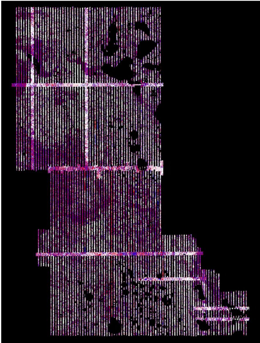
Figure 5 - QC block colored by vertical difference between swaths to check accuracy at swath edges by Axis Geospatial.
