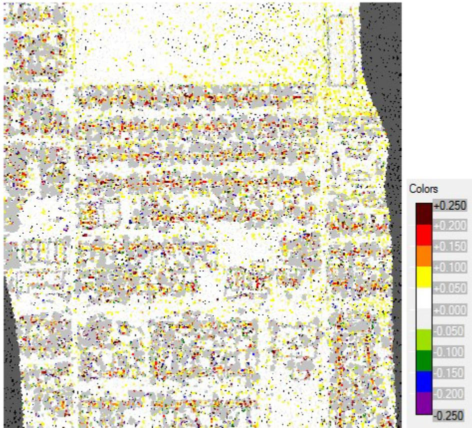
Figure 11- QC block colored by vertical difference between swaths to check accuracy at swath edges.
