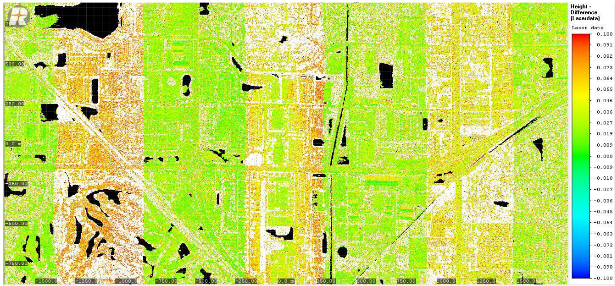
Figure 6. QC block colored by vertical difference between swaths to check accuracy at swath edges.
