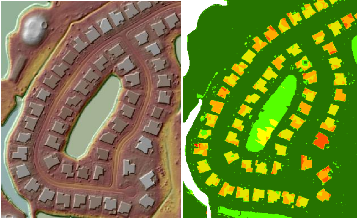
Figure 6 - The left image shows the final digital elevation models in Hillsborough County, with building rooftop heights represented. Elevation differences exist within building rooftop polygons, due to differences in breakline collection between Hillsborough County and FL Peninsular Pinellas County. The difference raster is shown on the right, displaying expected elevation differences between counties where buildings exist.
