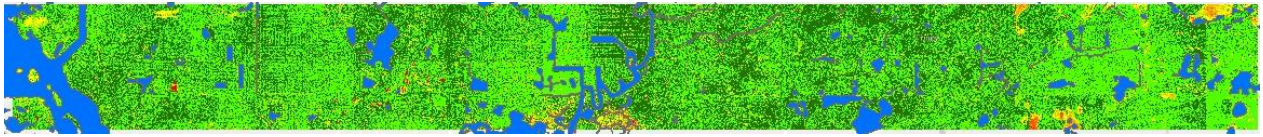
Figure 4 - Breaklined hydrographic features, shown in blue, were removed from statistical analysis generated from the difference raster as water levels may vary between the different lidar acquisition years.
