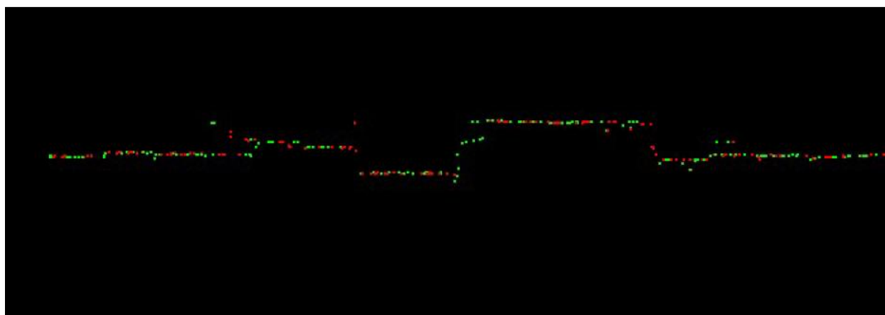
Figure 5a. Profile views showing results of roll and pitch adjustments by Airborne Imaging.
