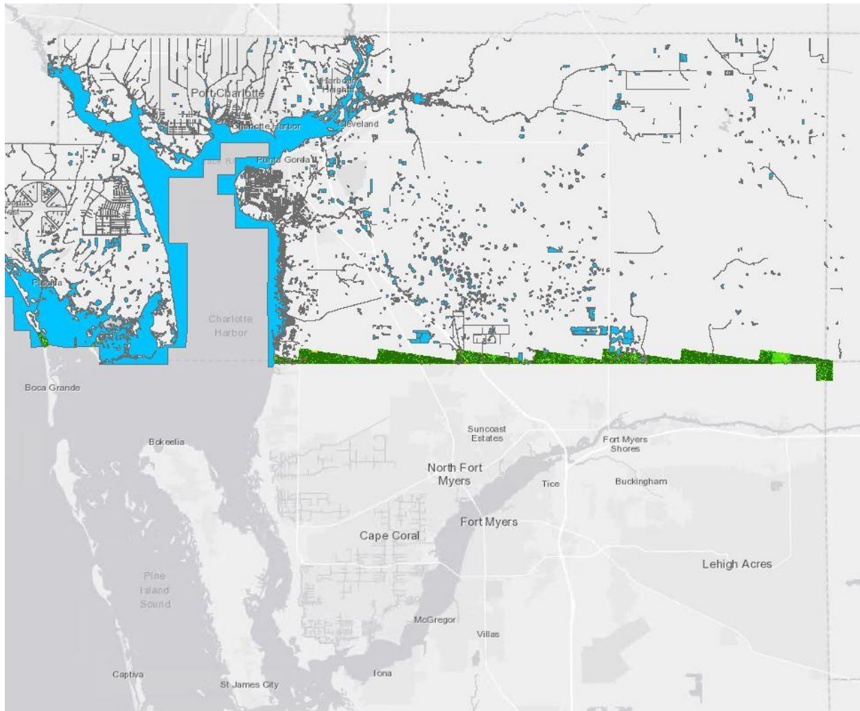
Figure 4-Breaklined hydrographic features, shown in blue, were removed from statistical analysis generated from the difference raster as water levels may vary between the different lidar acquisition years.
