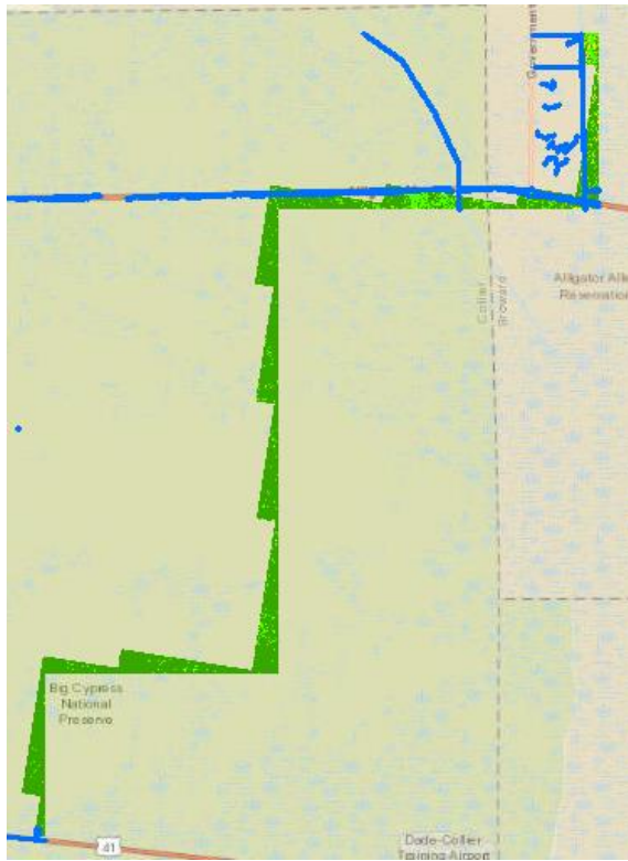
Figure 4-Breaklined hydrographic features, shown in blue, were removed from statistical analysis generated from the difference raster as water levels may vary between the different lidar acquisition years.
