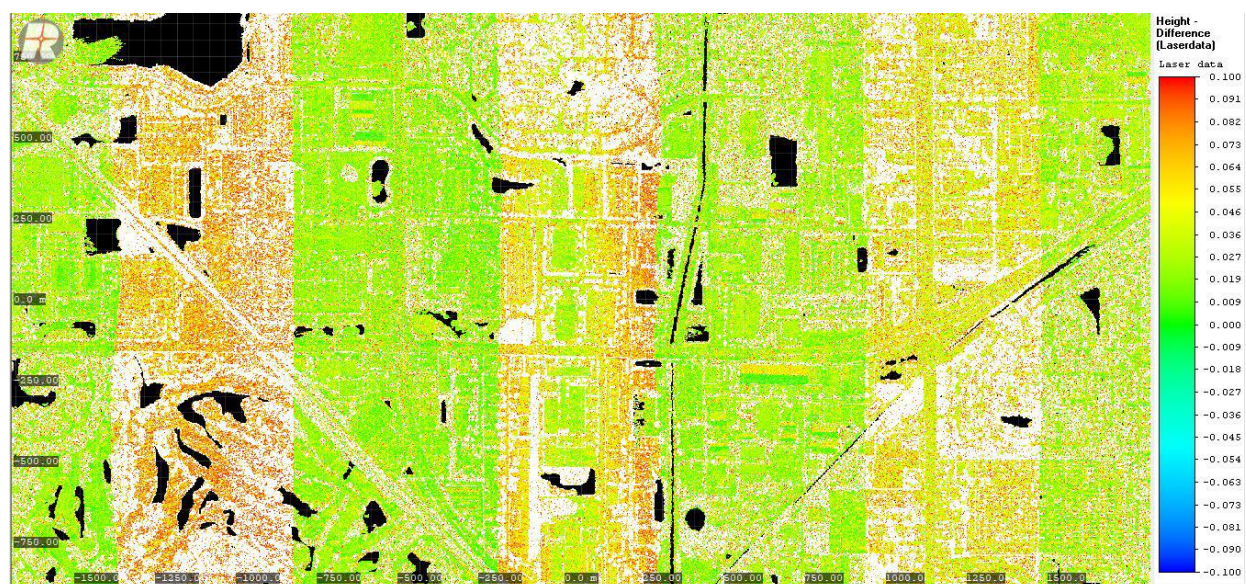
Figure 10. QC block colored by vertical difference between swaths to check accuracy at swath edges.
