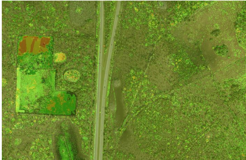
Figure 4-The image shows imagery overlaid with the difference raster (partially transparent). The largest values in the difference raster are over wetland/marsh areas, where there temporal difference of 2 years displays a difference in elevation.
