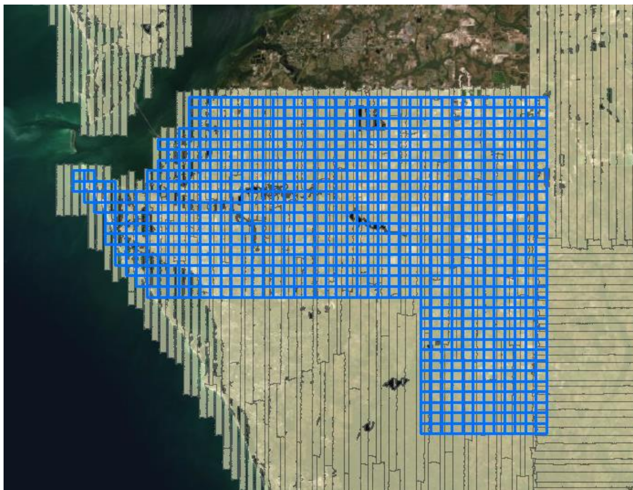
Figure 4. Lidar swath output showing complete coverage.
