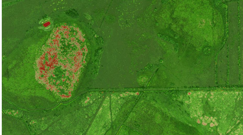
Figure 4- The image shows imagery overlaid with the difference raster (partially transparent). The largest values in the difference raster are over wetland/marsh areas, where there temporal difference of 2 years displays a difference in elevation.
