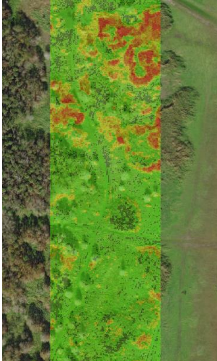
Figure 5-The image shows imagery overlaid with the difference raster (partially transparent). The largest values in the difference raster are over wetland/marsh areas, where a temporal difference of 7 years displays a difference in elevation.
