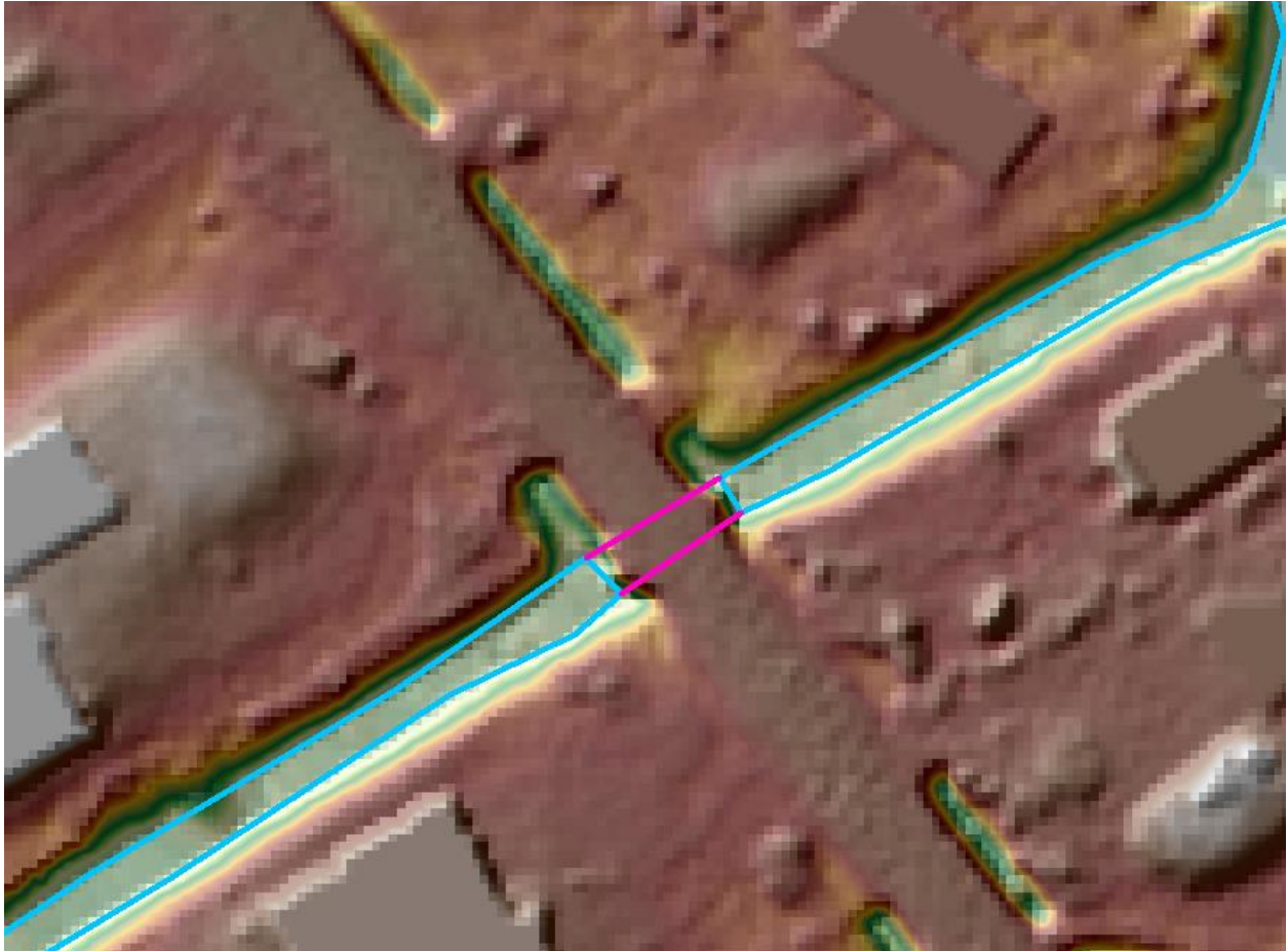
Figure 27- The image above shows proper placement of a connector (pink) across a culvert. The connector snaps to each end of the waterbody (blue).
