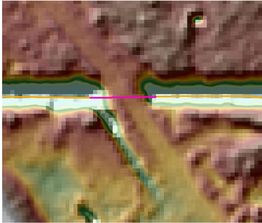
Figure 25- The image above shows proper placement of a connector (pink) across a culvert. The connector snaps to each end of the single line drain (yellow).
