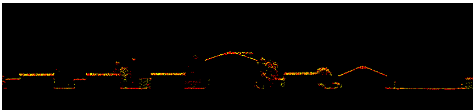
Figure 14—Horizontal Alignment. Two separate flight lines differentiated by color (Yellow/Red) are shown in this profile. There is no visible offset between these two flight lines. No horizontal alignment issues were identified.
