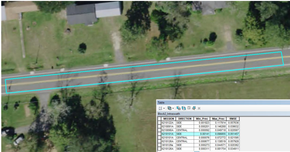
Figure 12—Example test polygon for intraswath testing, and its results
