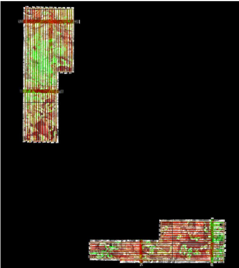
Figure 7: Area 1 & 2 QC block colored by distance to ensure accuracy at swath edges.
