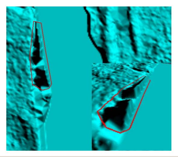
1 - smooth triangulation on tile seam @ 31° 15' 04.8555" N, 84° 49' 39.9932" W CORRECTED
