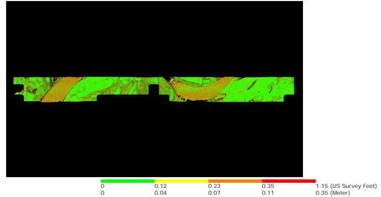
A maximum vertical separation cutoff has been applied to this graphic for the purpose of masking out disruptive features that do not show calibration issues between flight lines (e.g., trees, moving cars, etc.). This can be modified in the Color Options settings window.
