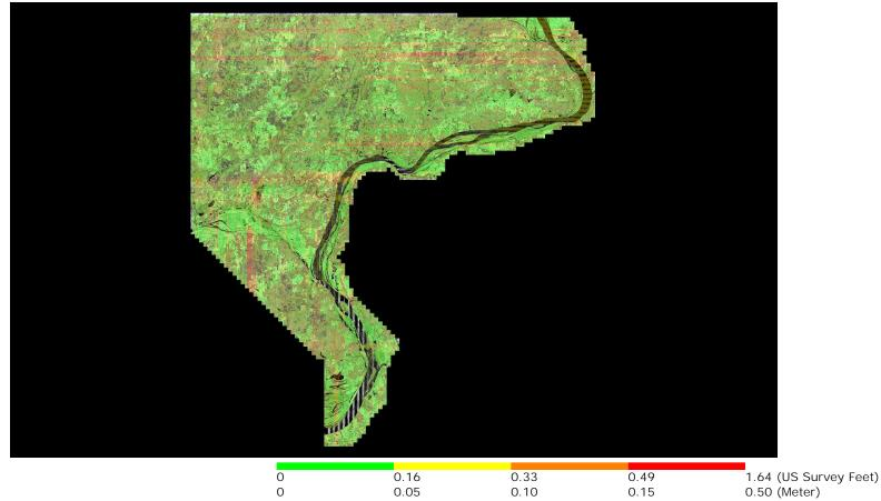
A maximum vertical separation cutoff has been applied to this graphic for the purpose of masking out disruptive features that do not show calibration issues between flight lines (e.g., trees, moving cars, etc.). This can be modified in the Color Options settings window.
