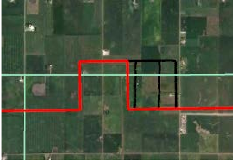
Figure 17: SURVTECH Block 3 LiDAR swath output showing complete coverage
