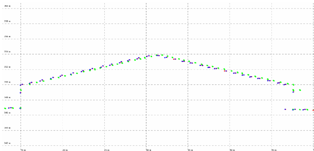
Figure 15: Profile views showing correct roll and pitch adjustments
